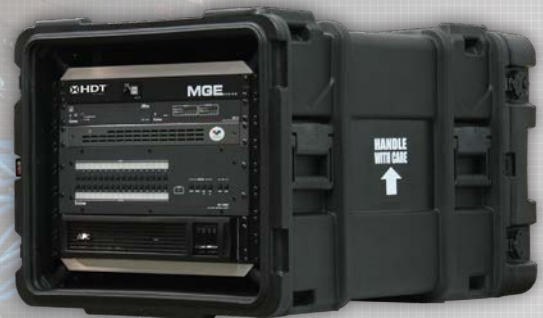
The standard AVDS has 16 inputs and 16 outputs, along with a quad splitter. The system can be expanded to 32 inputs and 16 outputs with three quad splitters.
