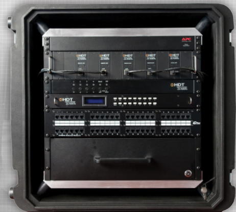
The standard AVDS has 16 inputs and 16 outputs, along with a quad splitter. The system can be expanded to 32 inputs and 16 outputs with three quad splitters.
